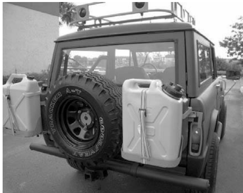
Fuel Storage Rack
